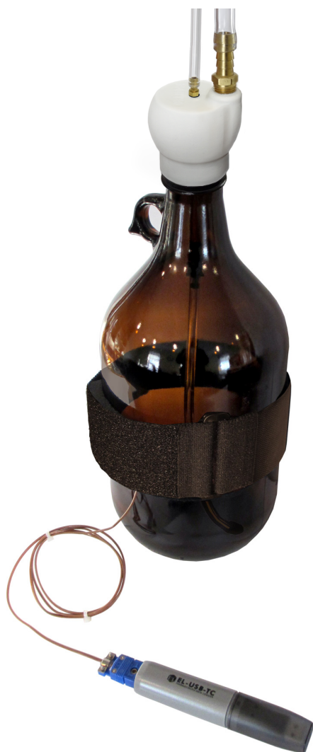
Fig. 4 Aerator and Bottle assembly with Temperature Logger
